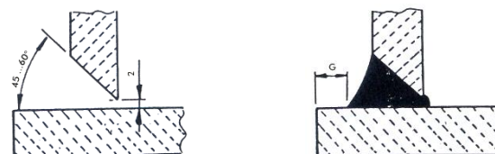
Joint to be welded
