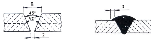
Separate joint to be welded
